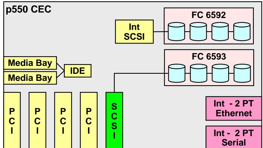
Note: The PCI SCSI adapter can be either RAID or non- RAID
