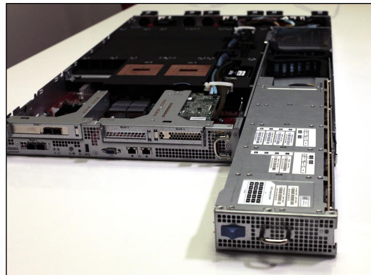
RackSpece Barreleys's : 2 socket POWER8 “Turrismo” 10 cores, 15 SSDs
